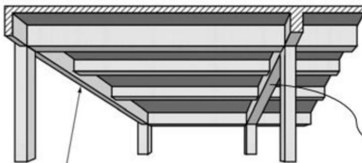
Design torque for this spandrel beam may be reduced because moment redistribution is possible
